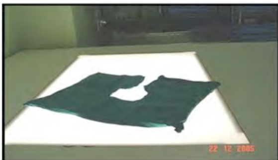
Figure 2. Illuminated table for checking
