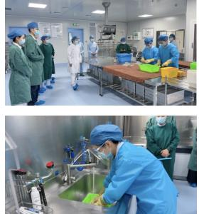
The staff in this area showed the collecting, classifying, dissembling, cleaning and disinfecting of used instruments in this area, as well as the principles and operation of washer-disinfectors. With a series of professional and rigorous cleaning and disinfection procedures, the instruments enter the inspection, packaging, and sterilization area.
