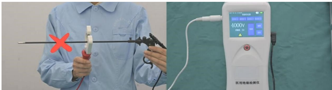
Workshop: Using Insulation Testers to inspect the Function of Electrically Powered Instruments
