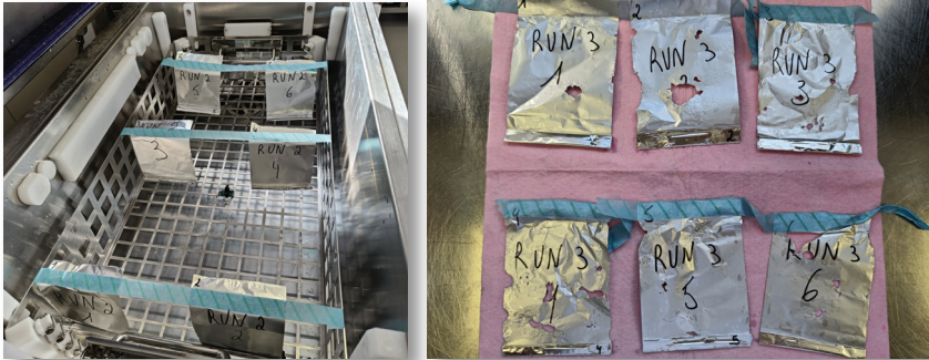
Figure 5: View of the perforation of aluminium strips by ultrasound waves
