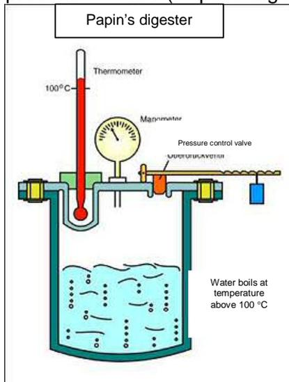
Water is heated in an enclosed space and allowed to boil until the space is filled with **saturated steam**. Under normal atmospheric pressure, steam can never be hotter than 100 °C, since it escapes. However, inside the pressure cooker the steam cannot escape and it reaches a higher temperature. At the same time, the pressure inside the pressure cooker increases, giving rise to **pressurized steam**.
