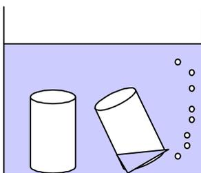
To ensure the presence of steam throughout the sterilizer and the devices to be sterilized, the air must first of all be removed because where there is air, there can be no steam, and vice versa. (Equally, where there is water, there can be no air, this is something we know from our daily working lives (see Fig.).
