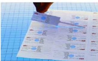
Treatment indicators show whether an item had been exposed to the sterilization process, but they do not provide any information on whether the sterilization process was properly executed. Hence the only insight gained is that the respective item had been exposed to the sterilization
