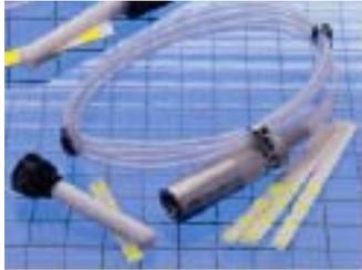
Special chemical indicators can be used for batch control. These provide information on whether steam had been in the chamber and in the devices to be sterilized and whether the (prescribed) temperature and hold time had been observed. The helix model has proved very useful to that effect (see Fig.). Here the chemical indicator is inserted into a process challenge device (PCD) which is connected to a 1.5 m long Teflon tube.
