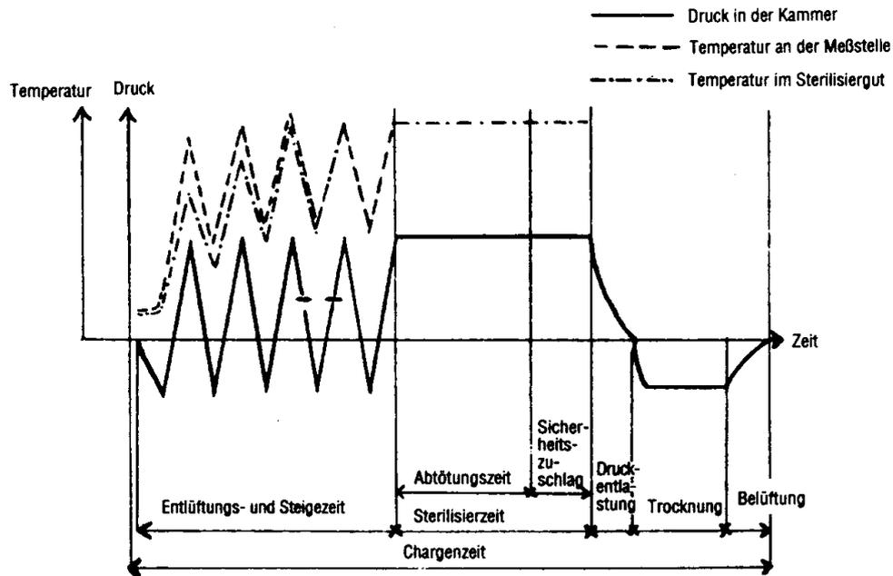
Fig.: Partial steps of the sterilization process (pulsed vacuum method)
