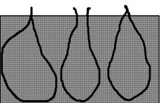
Too few items of flexible packaging in the sterilization tray Sealing seams, adhesive seams or adhesive sites could tear
