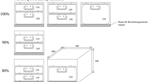
Two containers, with one placed above the other, with a height of 140 mm must not exceed a total height of 270 mm (technically possible by interlocking of the stacking mechanism)
